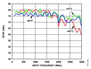
Figure 24. SFDR at 2.5GSPS vs. Temperature (Input Network in Figure 60 Used <2 GHz, Input Network in Figure 59 Used >2 GHz)
