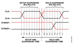
Figure 79. SYSREF± Edge Falls Within the Guardbanded Hold Time Window and Triggers an IRQ Error
