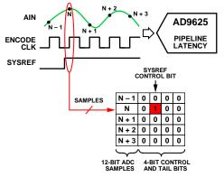
Figure 75. A SYSREF± Control Bit Can Be Used to Mark the Same Analog Sample that is Coincident with a Sampled SYSREF± Edge by CLK±
