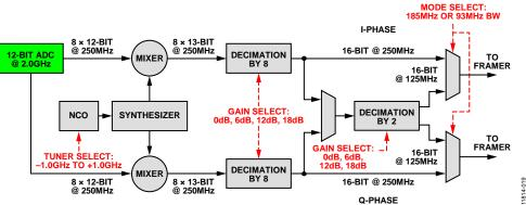
Figure 62. Digital Downconverter Block Diagram Operating at 2.0 GSPS
