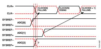
Figure 82. SYSREF± Case From Three ADCs Having Various Phase Delays Relative to the Falling Edge of the Encode Clock and will be Latched on Different Sample Clock Edges CLK±[N] or CLK±[N + 1]
