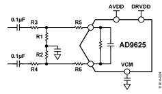
Figure 57. Recommended Front-End Network
