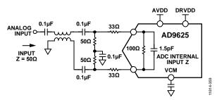
Figure 58. Input Network Example for Passive Balun with High Bandwidth
