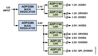
Figure 86. Power Supply Recommendation
