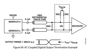
If there is no far end receiver termination, or if there is poor differential trace routing, timing errors may result. To avoid such timing errors, it is recommended that the trace length be less than six inches, and that the differential output traces be close together and at equal lengths.
