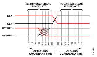
Figure 81. SYSREF± Edge Changes Phase Relative to the Encode Clock, Which can be Detected When the Edge Crosses Through the Guardband Setup Time
