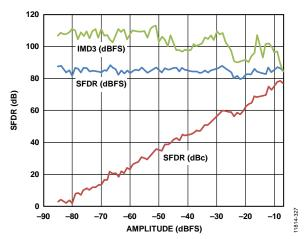
Figure 27. Two Tone SFDR and IMD3 vs. Analog Input Amplitude at 2.5 GSPS at 1800 MHz AIN
