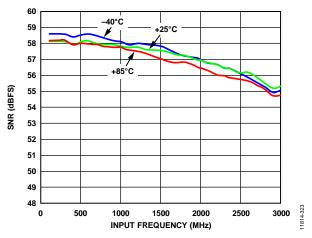
Figure 23. SNR at 2.5GSPS vs. Temperature(Input Network in Figure 60 Used <2 GHz, Input Network in Figure 59 Used >2 GHz)
