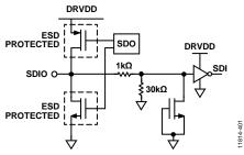
Figure 53. Equivalent SDIO Circuit
