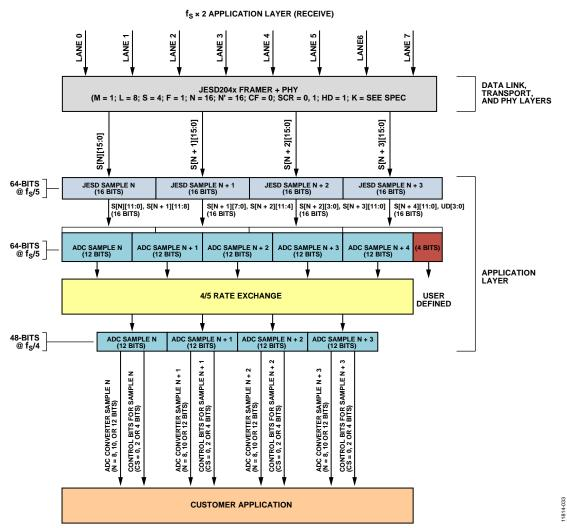
Figure 85.  $f_s \times 2$  Application Layer (Receive)
