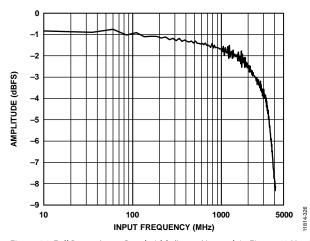
Figure 26. Full Power Input Bandwidth (Input Network in Figure 60 Used <2 GHz, Input Network in Figure 59 Used >2 GHz)
