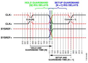
Figure 80. SYSREF± Edge Falls Within Both the Latest Hold Time Guardbanded of CLK±[N] and the Earliest Setup Time Guardband of CLK±[N + 1] and Triggers an IRQ Error
