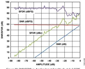
Figure 20. SNR/SFDR vs. Analog Input Amplitude at 2 .5 GSPS,  $f_{IN} = 241 \text{ MHz}$  at AIN
