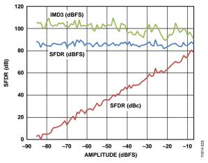
Figure 29. Two Tone SFDR and IMD3 vs. Analog Input Amplitude at 2.5 GSPS at 730 MHz AIN
