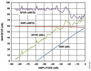
Figure 21. SNR/SFDR vs. Analog Input Amplitude at 2.5 GSPS,  $f_{IN} = 1811 \text{ MHz}$  at AIN
