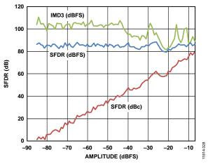
Figure 28. Two Tone SFDR and IMD3 vs. Analog Input Amplitude at 2.5 GSPS at 230 MHz AIN
