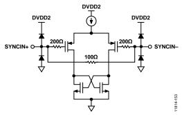
Figure 52. Equivalent SYNCINB± Input
