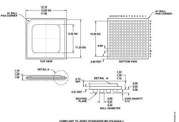
Figure 87. 196-Ball Ball Grid Array, Thermally Enhanced [BGA\_ED] (BP-196-2) Dimensions shown in millimeters
