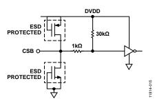
Figure 49. Equivalent CSB/PWDN Input Circuit
