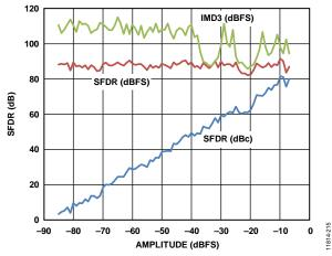
Figure 18. Two Tone SFDR and IMD3 vs. Analog Input Amplitude at 2.0 GSPS at 230 MHz AIN
