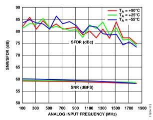
Figure 25. SNR/SFDR vs. Analog Input Frequency at Different Temperatures at 2.0 GSPS
