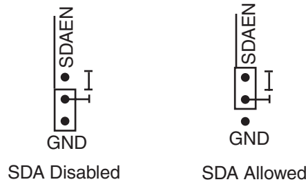
Figure 4-5. DC SDAEN Jumper Settings
